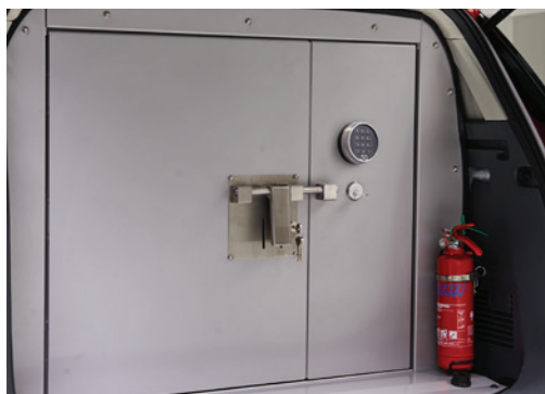
Cash box with double locking system
