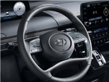
Semi-punched leather-wrapped steering wheel
