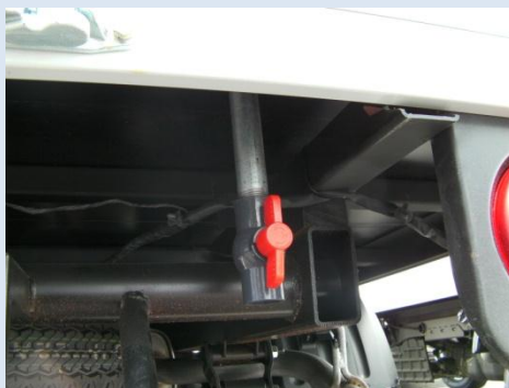
WATER DRAIN VALVE
